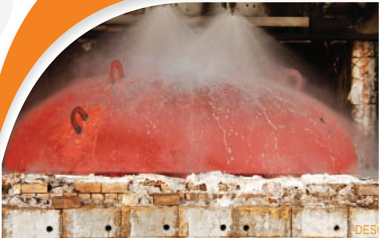
Solution annealing 4.5 dia. SS Dished end
