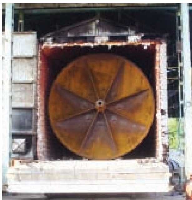
14 feet dia. MG roller PWHT
